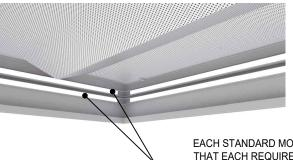
ROW OF LIGHTS IS NOTED BY A "UX-X" LABEL. THE "UX" CORRESPONDS TO AN INDIVIDUAL MODULE REFERENCED IN THE RCP AND THE "-1" AND "-2" CORRESPONDS TO THE ROW OF LEDS FOR THAT MODULE. EACH "UX-X" LABEL CORRESPONDS TO ONE (+ & -) LOW VOLTAGE WIRE TO BE FIELD CONNECTED TO URDC DRIVER CABINET AS PER THE MATCHING LABELS. EACH 100W DRIVER CAN POWER 1 ROW OF LEDS (ONE HALF OF A MODULE) AND EACH 600W DRIVER CAN CONTROL 6 ROWS OF LEDS (3 MODULES)
